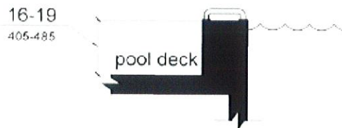
Figure 1009.4.2 Transfer Wall Height
